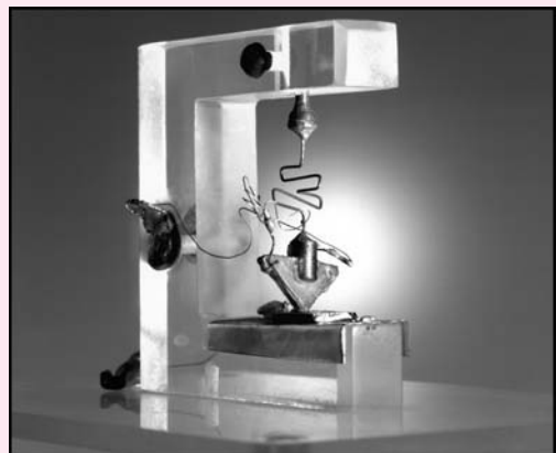
The first germanium bipolar transistor Reprinted with permission of Alcatel-Lucent USA Inc.
