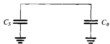
FIGURE 11.22 When the voltage of the selected word line is raised, the transistor conducts, thus connecting the storage capacitor C_S to the bit-line capacitance C_B .
