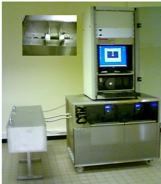
Figure 14.8. TSM experimental bench – External cooling technique
