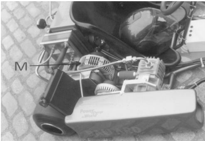
Figure 7.4 Small (10kW) DC ‘Lynch’-type DC motor, which is labelled M . This go-kart is fuel cell powered. The unit in front of the motor is the air pump, which is driven by its own motor – a smaller version of the traction motor
