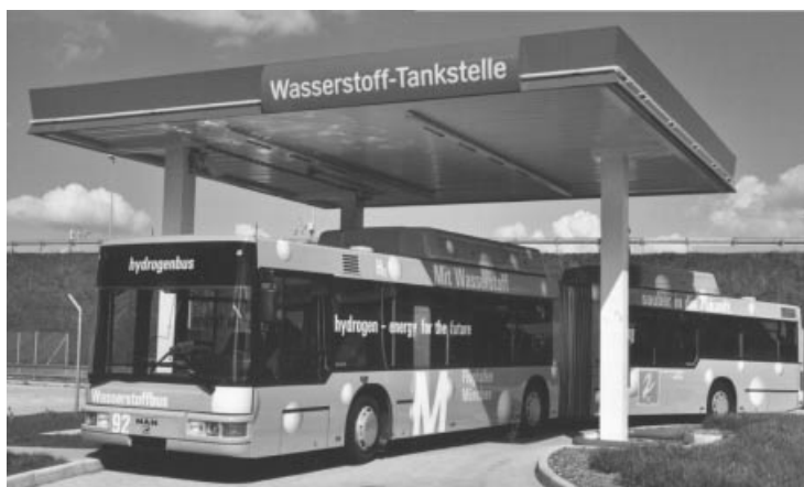
Figure 6.2 A hydrogen filling station. The bus in the picture is not electric, but uses a hydrogen-fuelled IC engine (Picture kindly supplied by MAN Nutzfahrzeuge A.G.)
