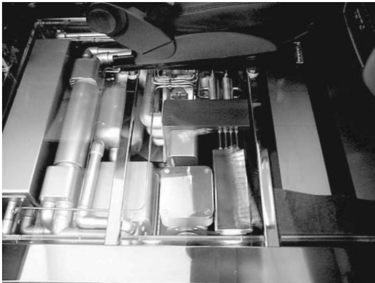
Figure 6.6 Packaging of the Nekar 5 methanol fuel processor
