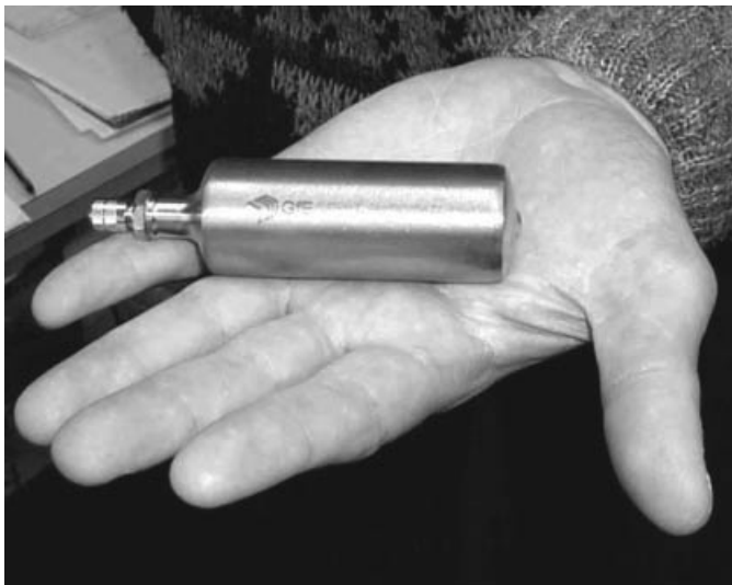
Figure 6.5 Metal hydride stores can be made quite small, as this example shows
