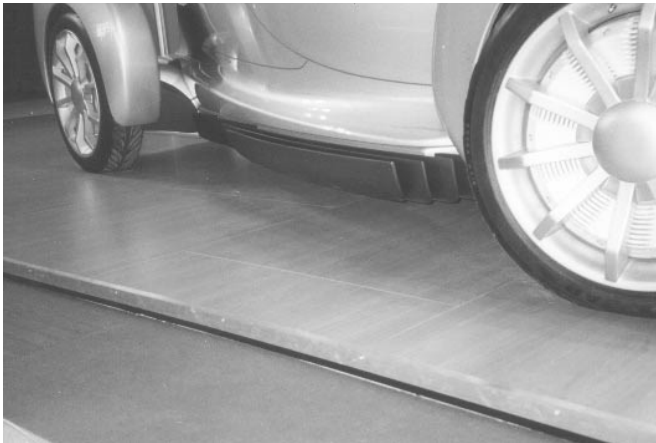
Figure 5.22 Solid metal cooling fins on the side of a GM Hy-wire demonstration fuel cell vehicle
