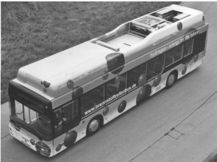
Figure 5.2 A fuel-cell-powered bus in use in Germany. Vehicles like this, used all day in cities, and refuelling at one place, are particularly suited to being fuel cell powered. (Reproduced by kind permission of MAN Nutzfahrzeuge AG.)
