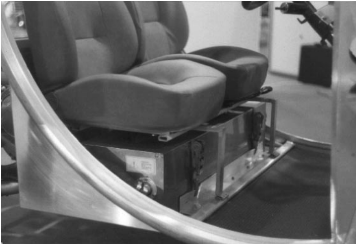
Figure 3.11 A commercial Zebra battery fitted neatly under the seat of an experimental battery electric vehicle by MES-DEA. The battery stores about 18 kWh of electrical energy
