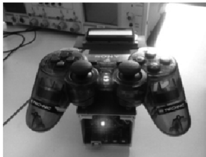
Figure 16.6. Manual control module
