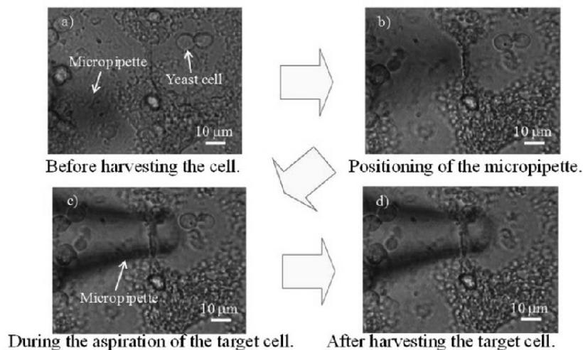
**Figure 2.8.** Single cell harvesting using semi-closed microchip
