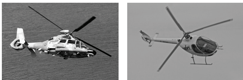
Figure 5.50. Helicopters of Different Tonnage With Different Control Systems: 5 Tons With Hydraulic System, and 0.6 Ton With Direct Mechanical System
