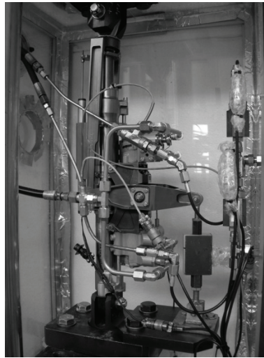
Figure 5.51. Servomechanism on a Characterization Test Bench (Source: Eurocopter)
