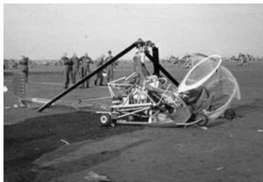
Figure 2.1. Disastrous Effects of Ground Resonance (photo: Ken Haan)
