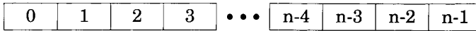
Figure 3.4 Arrays are the simplest data structure, allowing fast, random access (reading or writing) to the i^{\text{th}} element \forall i \in \{0 \dots n - 1\} where n is the number of elements in the array. Elements cannot be added or removed without copying the whole array.
