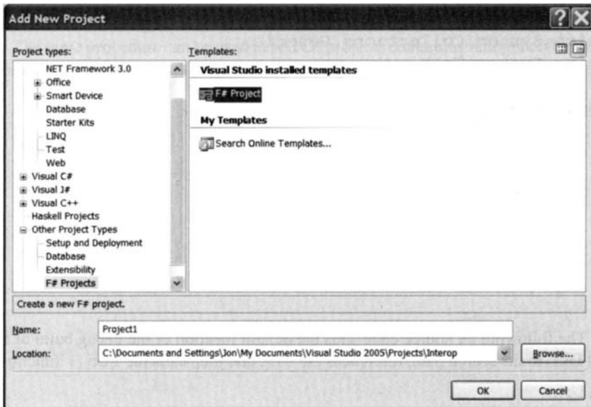
Figure 2.7 Creating a new F# project called Project1 also inside the Interop solution.
