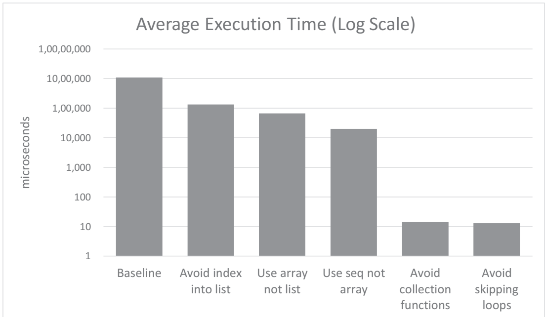
Figure 12-2. Impact of various improvements to collection usage on a log scale
