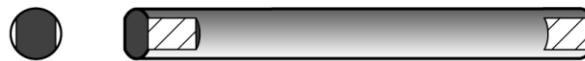
Figure 3.10. Parallel rectangular surfaces at each end of each cylinder are obtained by milling
