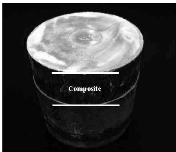
Figure 3: A squeeze cast magnesium matrix composite (AM60/Al 2 O 3 ).
