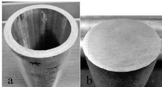
Fig. 4. (a) 13.34 cm OD extruded tube with 1.27 cm wall thickness, (b) 12.07 cm OD extruded rod.
