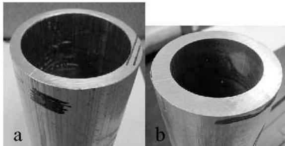
Fig. 3. Extruded tubes (a) 7.62 cm OD, 0.635 cm wall thickness, (b) 8.89 cm OD, 1.27 cm wall thickness
