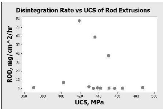
**Fig. 7.** Disintegration rate vs. rod UCS.
