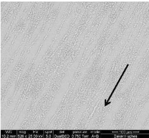
Fig. 11. SEM image of extruded S2. Direction of extrusion is depicted by arrow.
