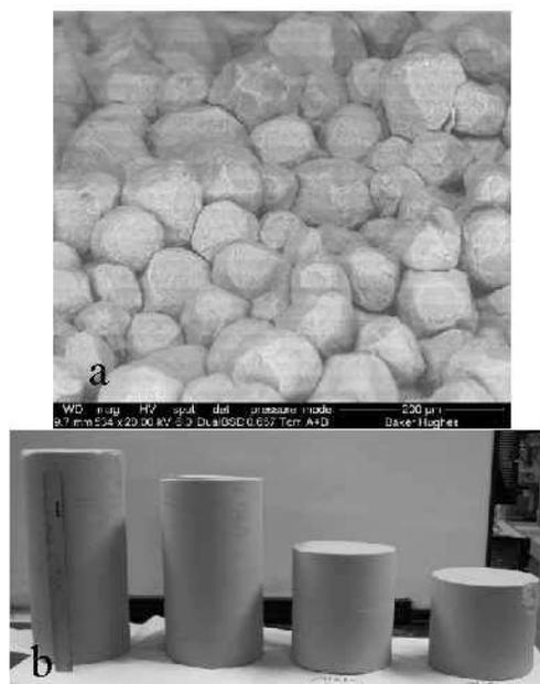
**Fig. 2.** Green preform of (a) powder, (b) billets.
