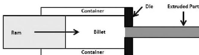
**Fig. 1.** Extrusion press diagram used for DMMC extrusion.
