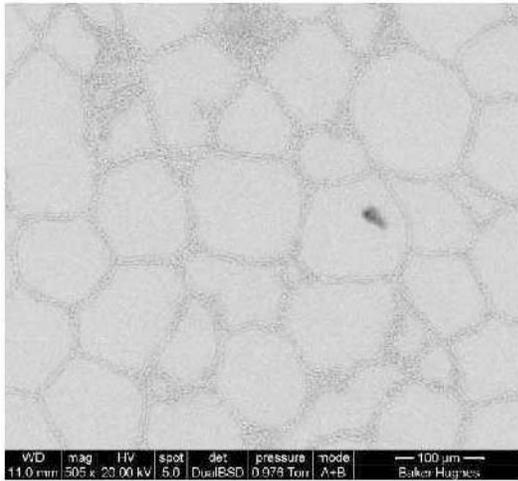
Fig. 10. SEM cross-section of forged S2.
