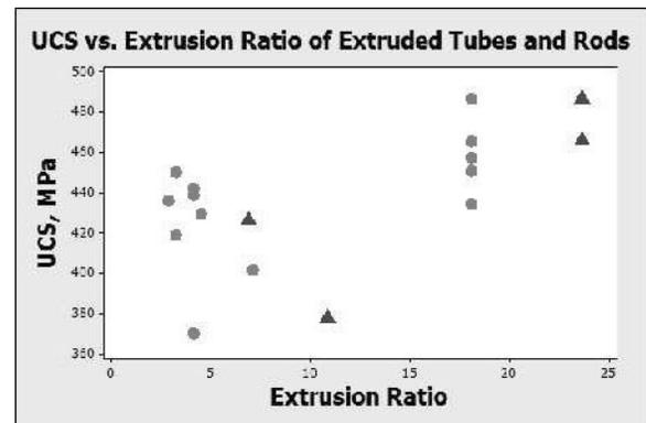
**Fig. 9.** UCS and extrusion ratio of extruded rods and tubes.
