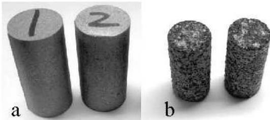
**Fig. 6.** Example of sample coupons of extruded parts (a) prior to testing and (b) after exposure to brine at 93.3°C .
