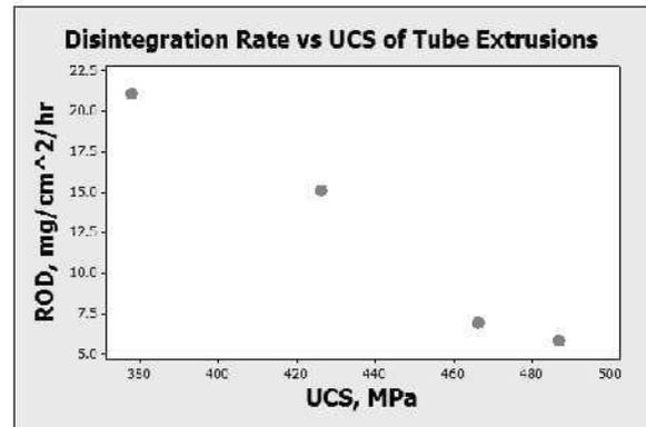
**Fig. 8.** Disintegration rate vs. tube UCS.
