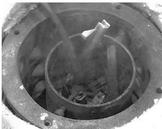
Fig. 3. The remaining tar and char on the surface of magnesium alloy scraps during decomposition of polyurethane scraps by heating at 400°C in air.
