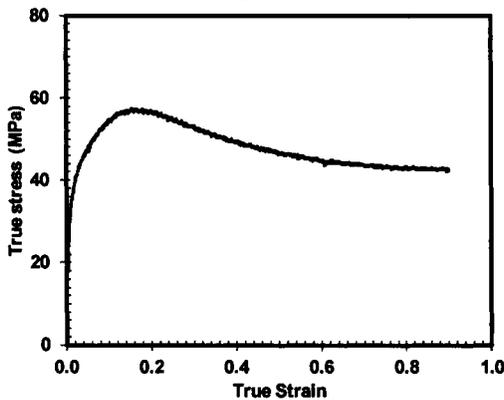
Figure 5: Flow behavior of Mg-3Al-2Sn alloy at 300  $^{\circ}\text{C}$  and strain rate of 0.01  $\text{s}^{-1}$ .
