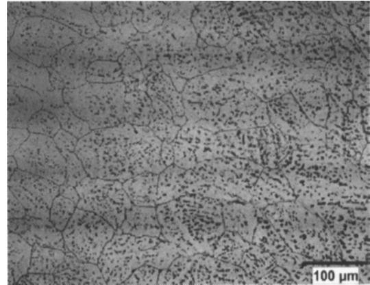
Figure 2: As-cast optical microstructure of Mg-3Al-2Sn alloy
