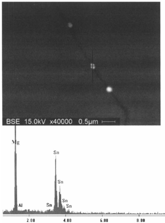
Figure 9: Precipitate formation at DRX grain boundary and EDS qualitative analysis of the precipitate.
