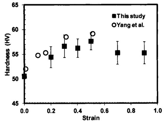
Figure 10: Variation of room temperature hardness with strain.
