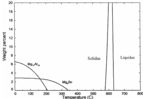
Figure 1: Equilibrium phase fraction of Mg-3Al-2Sn alloy predicted by FactSage.
