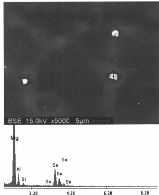
Figure 3: As-cast SEM microstructure of Mg-3Al-2Sn alloy and EDS quantitative analysis of the precipitates.
