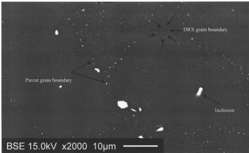
Figure 8: Grain boundary pinning effect by precipitates (300 °C, strain rate  $0.01\text{s}^{-1}$ , strain 0.9).
