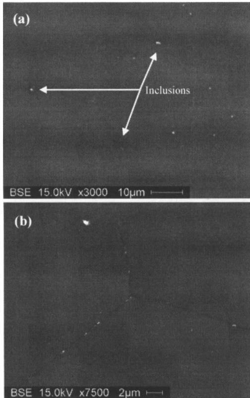
Figure 4: Homogenized and aged microstructure of Mg-3Al-2Sn alloy (a) Homogenized (b) Aging at 300  $^{\circ}\text{C}$  for 10 min and quenched
