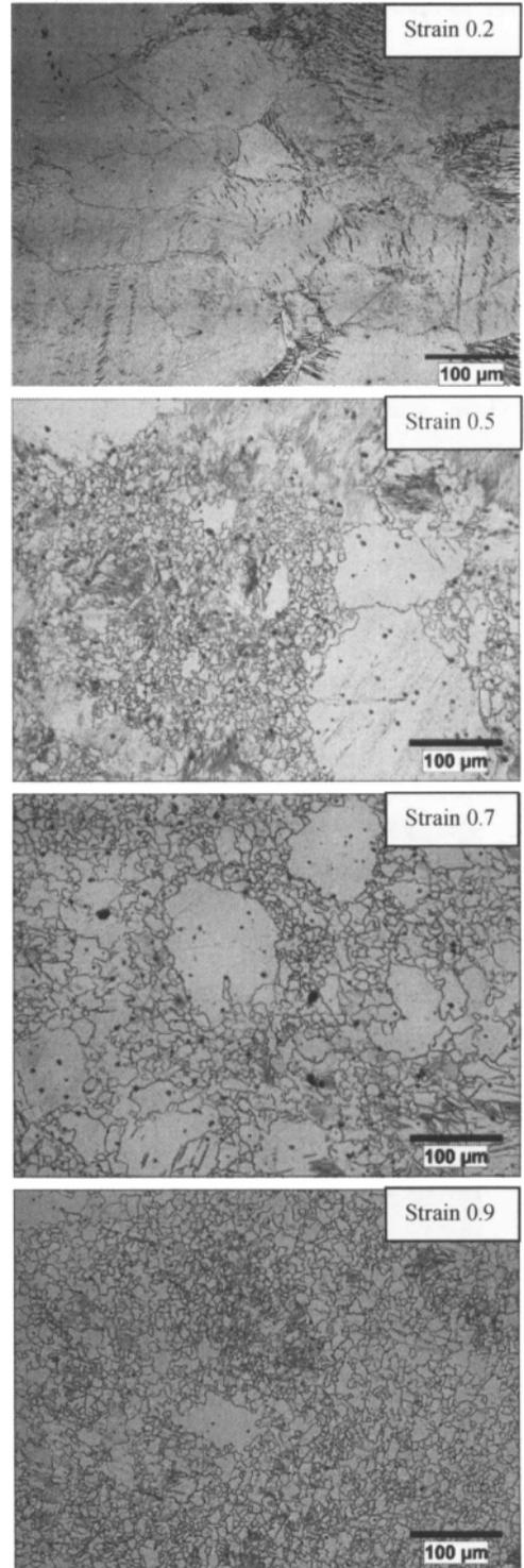
Figure 6: Microstructure evolution with different amount of deformation
