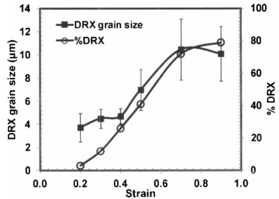
Figure 7: Variation of % DRX and DRX grain size with different strain.
