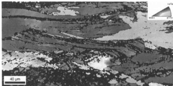
Figure 4. EBSD map (referring to the ND) after rolling at 450 °C (followed by annealing at 400 °C for 3 min) showing horizontal bands in basal parent grains. The maps show the RD-ND plane with the RD being horizontal.
