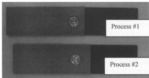
Figure 2. Representative lap-shear coupons produced from process #1 and process #2.
