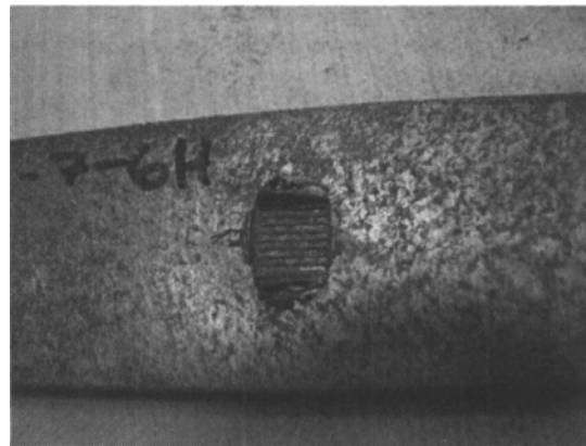
Figure 2. Appearance of AZ31 surface after 1 cycle of corrosion test.
