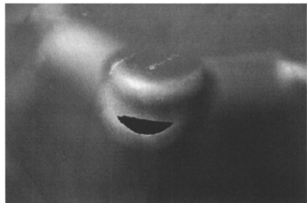
Figure 13 – Photograph showing the failure of an AZ31B shear rolled sheet formed at a faster rate
