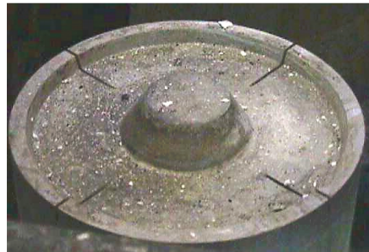
Figure 4 – Deformed center cone on stool cap made from aluminum.
