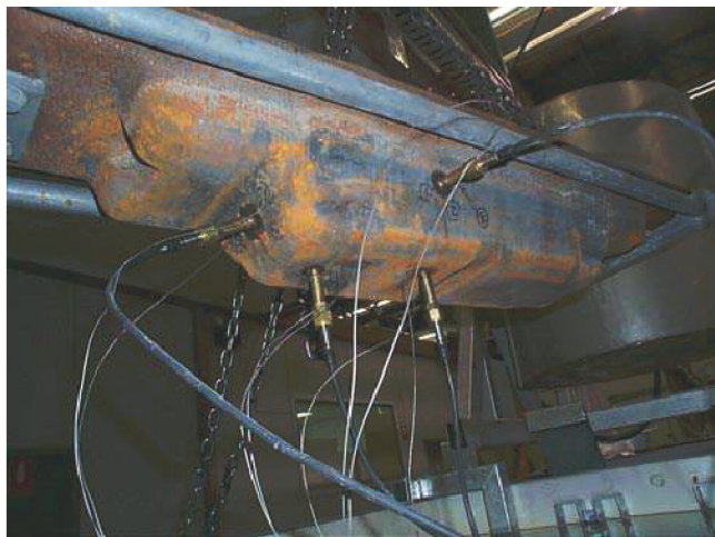
Figure 2 LVDTs and thermocouples inserted in mold on ingot rig to measure air gap formation, solidification times and heat flow [9].
