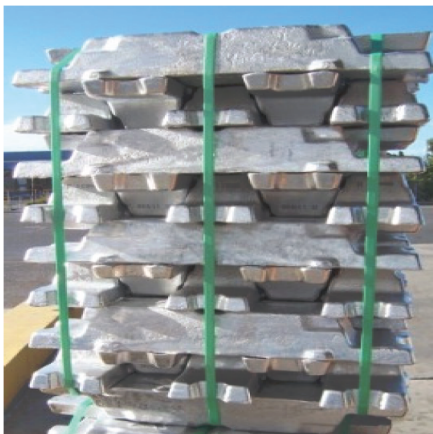
Figure 4 Plastic strapping used on 23 kg bundle.
